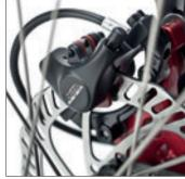
Speedy wheels need strong stoppers. For us, this means reliable hydraulic disc brakes. They not only offer superior braking power: unlike cable-actuated brakes, they are extremely responsive and provide perfect modulation.
