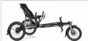
The concept for relaxed mobility The seat height, adjustable from  $22\frac{1}{2}$  to photo) is now compatible with the 25 inches (57-63 cm), gives you an excellent view of traffic, and the new, rear-suspension frame guarantees maximum stability, safety, and comfort, with a relaxed, intuitive ride. And as a bonus: cargo transport has never been so easy.
