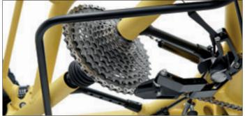
Special uses - special components The use of derailleur gears on trikes with full suspension has always been a challenge: when the suspension compresses, the standard, low-hanging derailleur cage can come in contact with the ground. This is why we decided to develop our own derailleur system. It
