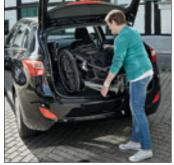
rear portion of the trike folds down and forward. The "LEPUS pack" is only about three feet (1 m) long with the front wheel and fits into almost any combact car.
